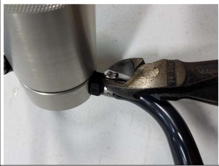
Once hoses are removed, you will need to move the 90° fitting to point downward. Use 18mm box end wrench to do this, or long screwdriver shoved into the end of the fitting to move it.
